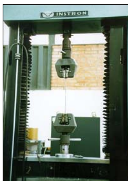
Figure 7 - Aluminum and steel wires vertical traction machine of 10 tons view.
