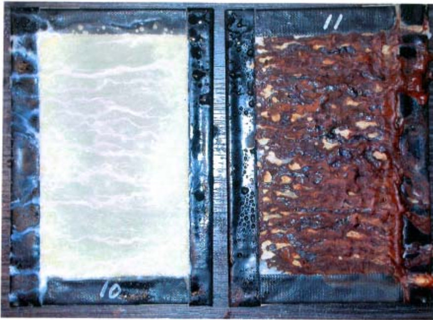
Picture 19. Plates 10, 11 after 2212 hours exposure
