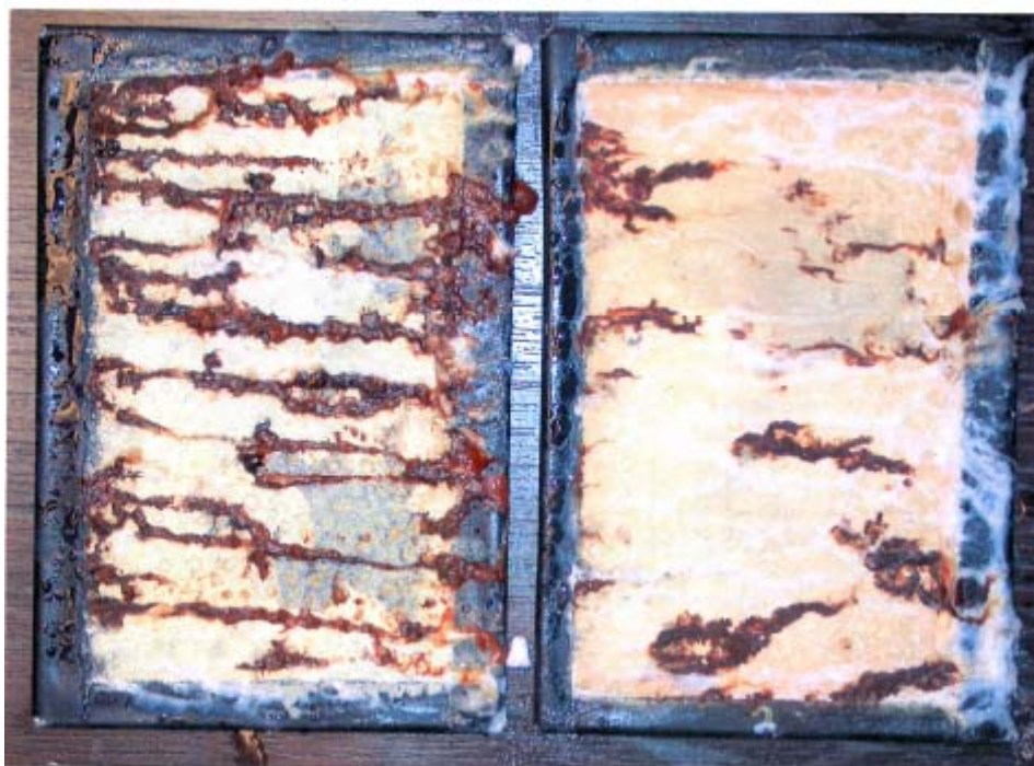
Picture 14. Plate 1, 2 after 2212 hours exposure
