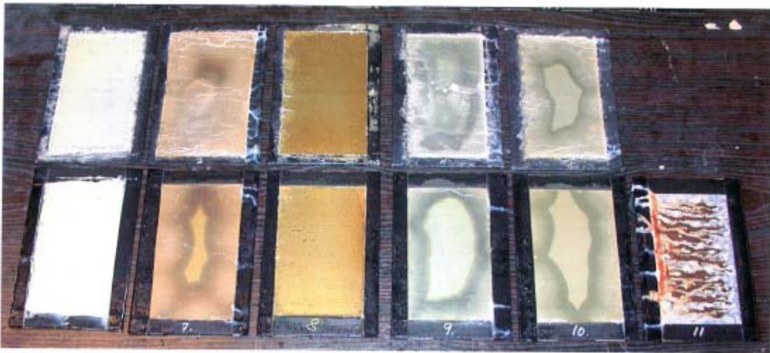
Picture 7. Overview over zinc coated steel plates after 511 hours exposure
