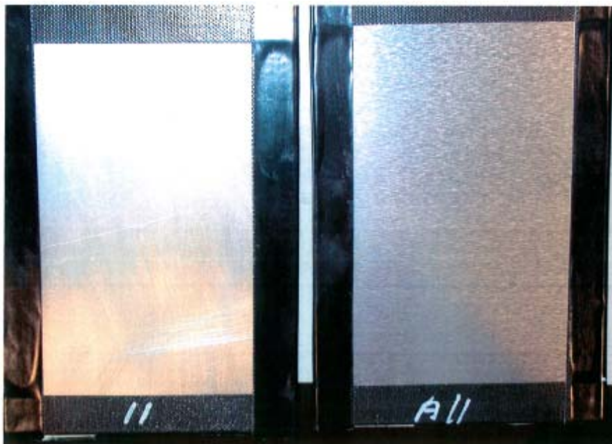
Picture 6. Reference plates before exposure
