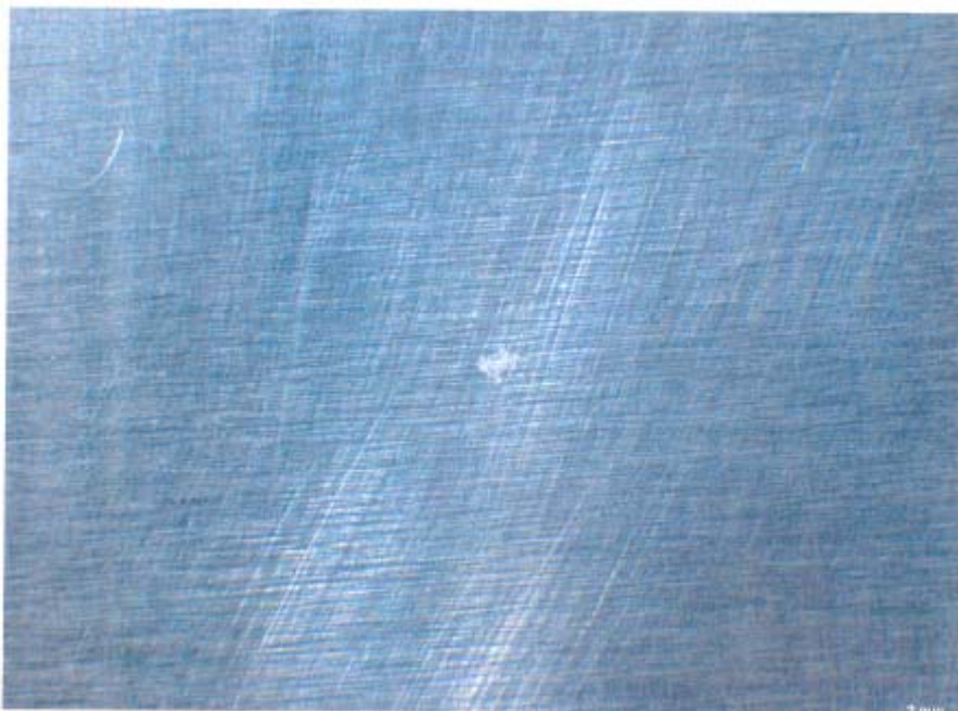
Picture 20. Stereo microscope. Plate A1 after 2212 hours exposure In the middle of the picture, a small superficial corrosion attack is visible after removing the grease film. Note that the magnification is specified in right bottom corner
