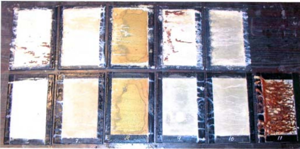
Picture 12. Overview of all zinc coated steel plates after 1467 hours exposure
