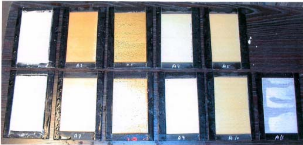
Picture 13. Overview of all aluminum plates after 2212 hours exposure
