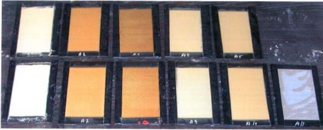
Picture 11. Overview of all aluminum plates after 1467 hours exposure
